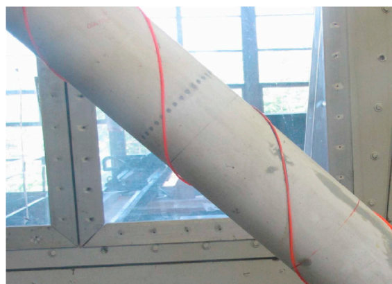
Fig. 2. The side of the cable with the helical fillets normal to the oncoming flow near ring 2 for a cable inclination of 45° and a cable rotation of -25°.
